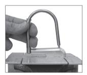
Clamp the functional unit by using a vice with braces. Position the narrow end of the assembly aid for the cover plate below the ball of the functional unit and fix the plastic-sheathed side on the upside of the spring duct by tensioning the spring.
