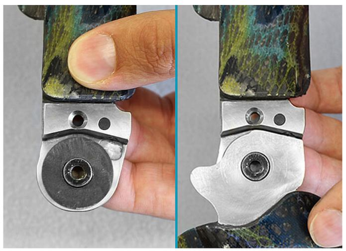
Place the second sliding washer onto the joint's upper part and mount the system stirrup while still fixing the bearing nut.
