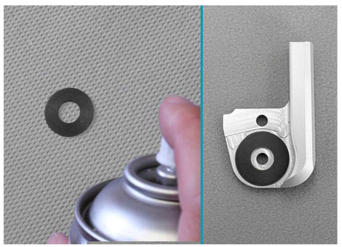
Apply spray adhesive to one side of the first sliding washer and adhere it to the cover plate. Continue by greasing the other side of the sliding washer slightly with orthosis joint grease.
