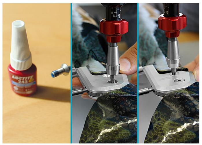
Secure both screws with LOCTITE<sup>®</sup> 243 medium strength and the torque corresponding to the system width. Let the adhesive harden (final strength after approx. 24 hours). Insert the ball, the pin and the spring into the spring duct and turn in the pressure screw as far as possible. *Note: Mind the* safety data sheet when using LOCTITE<sup>®</sup> 243 medium strength.
