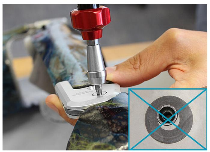
If you have damaged the sliding washer during the assembly of the cover plate (you would hear a soft cracking), remove the particles and place a new sliding washer.
