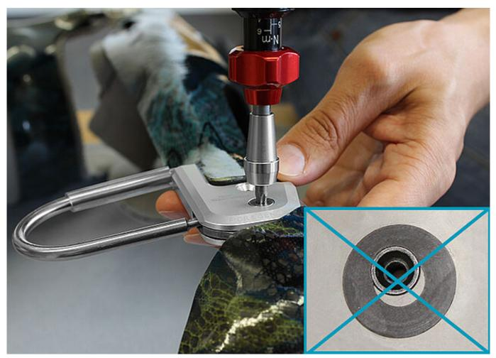
If you have damaged the sliding washer during the assembly of the cover plate (you would hear a soft cracking), remove the particles and place a new sliding washer.
