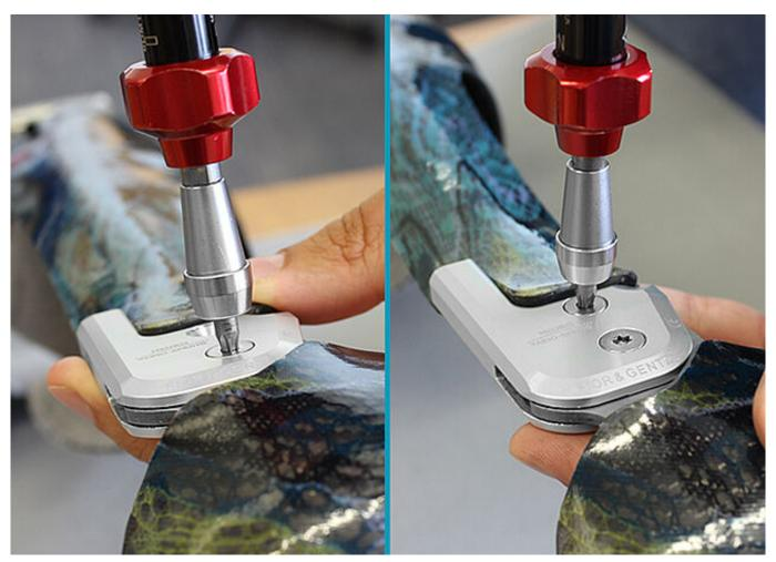
Mount the cover plate. Turn in the first countersunk flat head screw (axle screw). Continue with the second countersunk head screw using the corresponding torque while still fixing the bearing nut. *Note: You will find the appropriate torque (Nm) on the cover plate of the system joint or in the instructions for use.*
