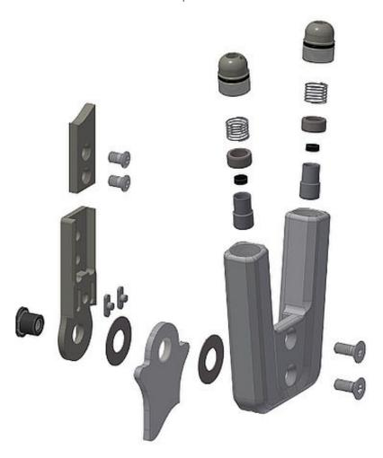
Clean the system joint. In order to clean the threads in the cover plate, use the Super Clean LOCTITE® 7063 to remove any insulating wax residues.
