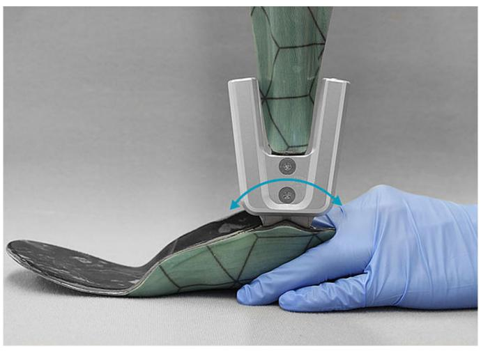
Bring the system joint in plantar flexion/dorsiflexion. Any present spring units should move by compression only. At a high spring force, it might be impossible to cause any movement manually. If the system joint still runs idle, carefully screw the posterior alignment screw further in.
