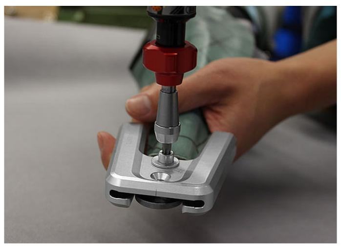
Use the delivered cover plate pressing aid to press the cover plate with the joint's upper part. Tighten the pressing screw with the corresponding torque.
