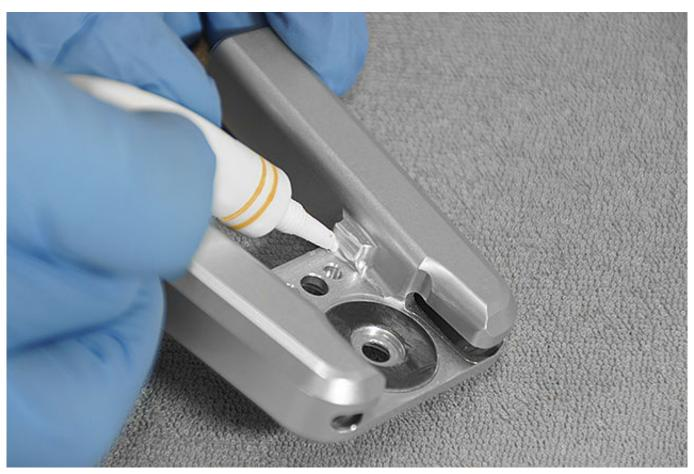
Grease the contact surfaces of the cover plate with orthosis joint grease to prevent friction noises between cover plate and joint's upper part.
