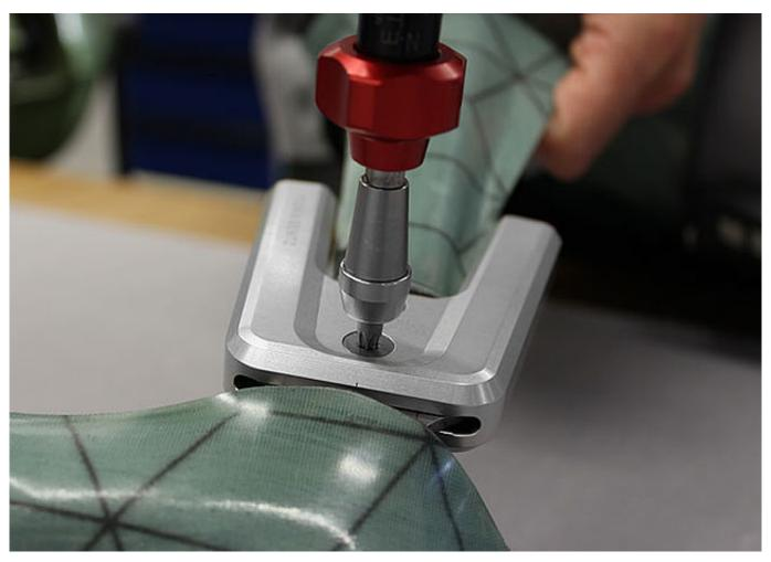
Screw in the second countersunk flat head screw (axle screw) with the torque which corresponds to the system width while fixing the bearing nut from the backside with one finger.
