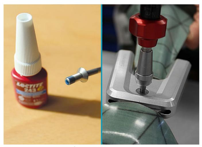
Secure both screws with LOCTITE  $243^{\circ}$  medium strength and the torque corresponding to the system width. Let the adhesive harden (final strength after approx. 24 hours).
