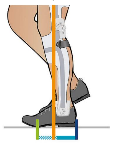
The loading line should run through the front half of the supportive area. The supportive area in mid stance is defined by the heel lever and the rolling-off area. For the course of the loading line to be correct, measures ought to be taken, such as a posterior offset of the heel or an anterior offset of the mechanical rolling-off area.
