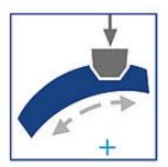
A flexion stop/a flexion limitation is realised through the joint's locking. It is either permanently locked or locks in swing phase. A flexion limitation through a stop, which is limiting the range of motion, is only useful in exceptional cases and does not serve stability while walking but is meant to prevent torn tendons or the like.
