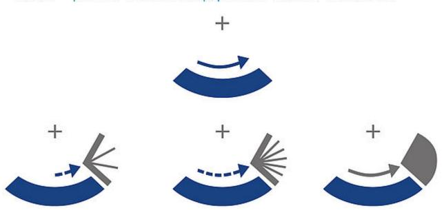
Similar to the dorsiflexion stop, the plantar flexion stop can be realised in a number of ways and the effects differ, depending on the gait phase. Instead of a plantar flexion stop, this is often referred to as a foot lifting effect.
