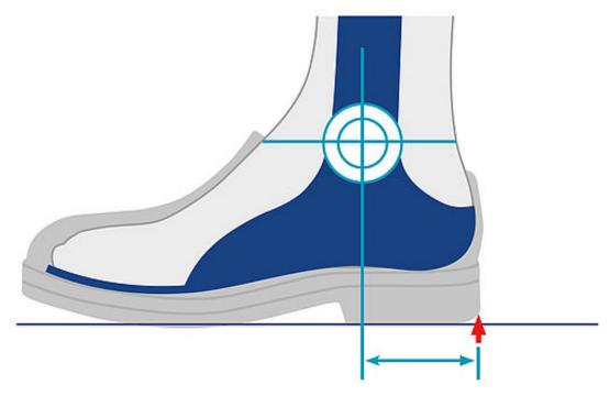
The mechanical heel lever represents an axis. The foot rotates around this axis. In addition, the heel lever limits the stance area (supportive area) proximally. The anatomical heel lever can significantly differ from the mechanical one. The heel lever affects the gait phases initial contact, loading response, early mid stance, mid stance and late mid stance.
