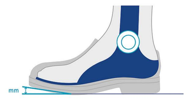
The toe spring affects the gait phases terminal stance, pre swing and initial swing. It does not affect any other phases. The effects on the gait phases must always be considered in regards to the dorsiflexion stop and the forefoot construction.
