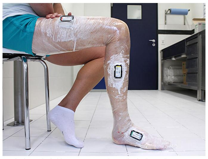
Form the plaster and embed the sensors in it. Repeat this procedure for all required sensors.
