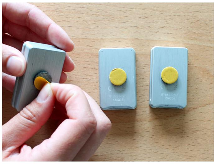
Connect the sensors to the operator device. Remove the protective foil on one side of the glue dots to attach them to the sensors' centre.
