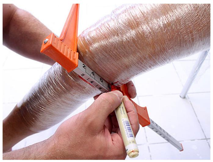
You can mark the position of the mechanical pivot point in ap direction with the callipers. Mark the x measurement by using the printed configuration result.
