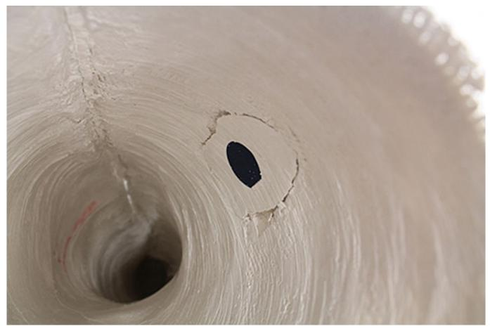
The cast surface is level on the inside and you can only see the glue dot from the sensor. Like this, you avoid that the cast loses its form.
