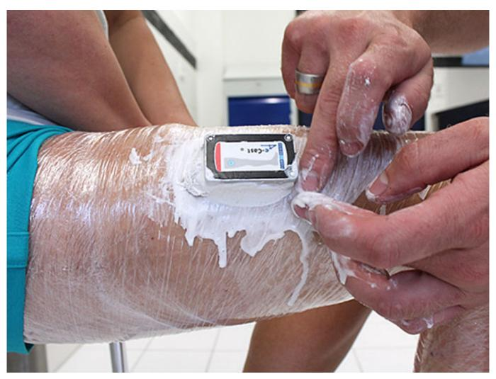
Put the prepared longuettes under the sensors for stabilisation purposes. For a positive fit between sensor and leg, it is necessary to fill out the space completely with plaster. Make sure not to push the sensors away from the leg because otherwise they do not stick optimally on the film.
