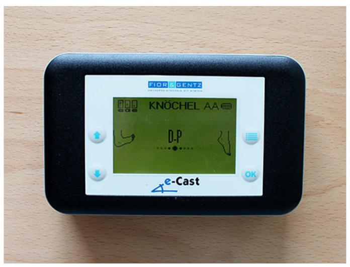
The operator device indicates when the current position differs from the saved one. The dot on the display moves towards plantar flexion (P) or dorsiflexion (D) if the position differs into the corresponding direction. When the dot is in the **middle**, the position matches the saved one. If you have activated the display of pronation and supination in the menu Settings, you can reconstruct this position by shifting the knee in mediolateral direction.
