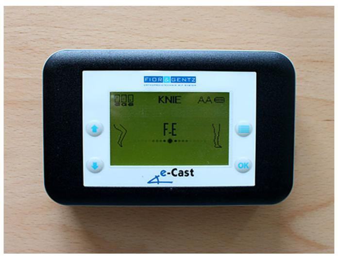
The operator device indicates when the current position differs from the saved one. The dot moves towards extension (E) or flexion (F) if the position differs into the corresponding direction. When the dot is in the **middle**, the position matches the saved one. If you have activated the display of varus and valgus in the menu Settings, you can reconstruct this position.
