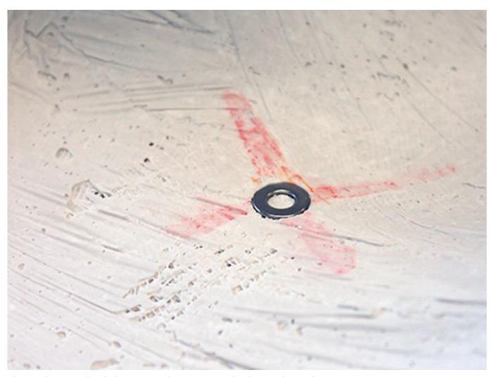
The washer can clearly be seen in the cast. It marks the mechanical pivot point.
