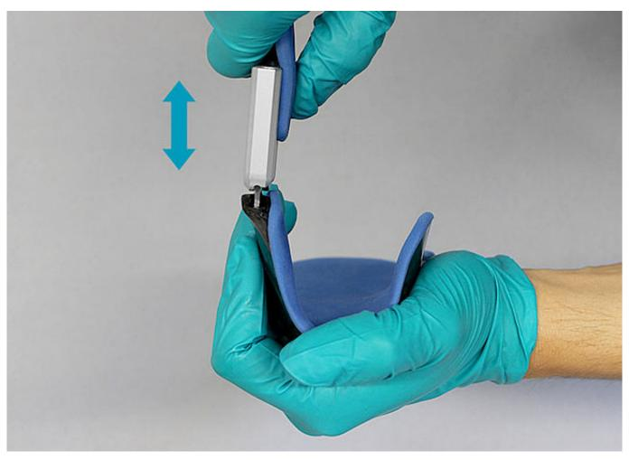
Check if there is play around the axis. If there is play, the bearing nut and the repair bushing should be replaced or inserted if necessary.
