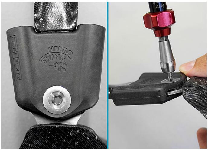
Disassemble the system joint completely. Clean all component parts and check them carefully.
