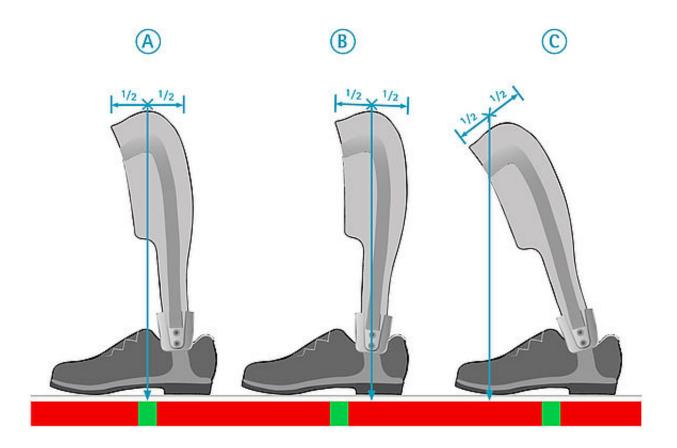
Check the alignment on the workbench considering the shoe pitch:
