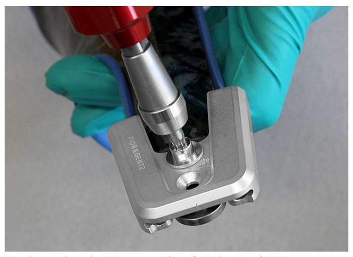
Mount the cover plate to the joint's upper part without adhering them. Press the joint's upper part to the cover plate as described in the manual. Continue assembling the joint as usual.
