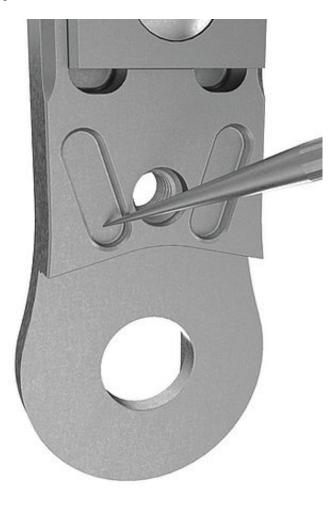
Clean the grooves of the joint's upper part **thoroughly**, otherwise the feather keys with pin cannot be mounted correctly. This is important, as incorrectly mounted feather keys with pin are very hard to remove.
