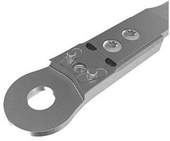
Remove the assembly/lamination dummy. Press the feather keys with pin carefully to the joint's upper part in a vice with plain jaws until the feather keys with pin are flush with the joint's upper part.
