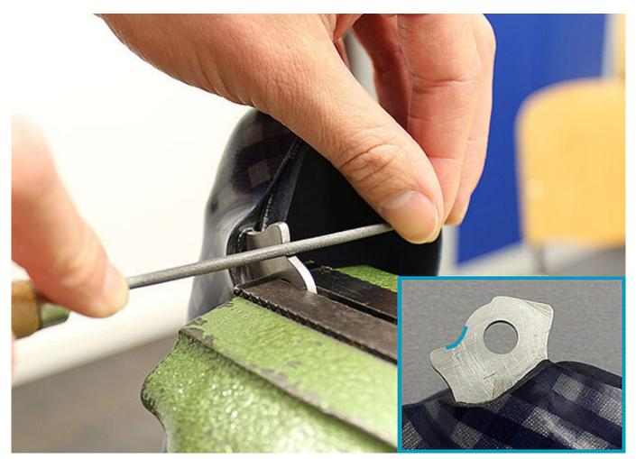
Grind the system stirrup with a round file up to the laser line.
