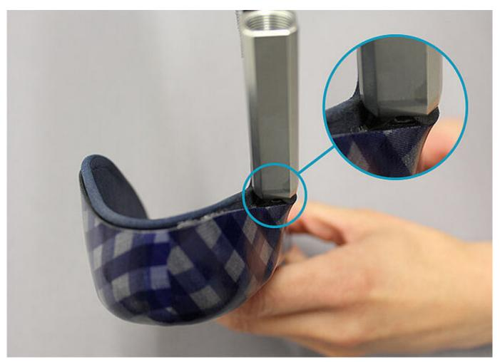
Also check if the back of the cover plate fits well and adapt the laminate, if necessary.
