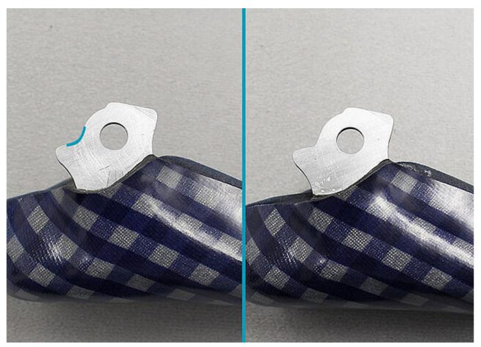
After having ground the part marked with a line, the system stirrup looks as shown on the right picture. *Note: Make sure not to create any predetermined breaking points when grinding*
